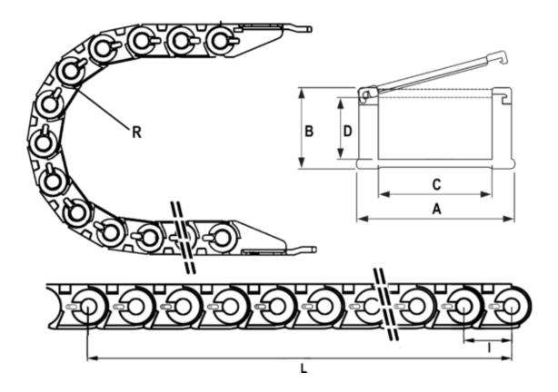
Full length = 990mm Inside Height = 19 Inside Width = 50 Link Length(Pitch) = 30 Outside Height = 26 Outside Width = 64 Radius = 100
